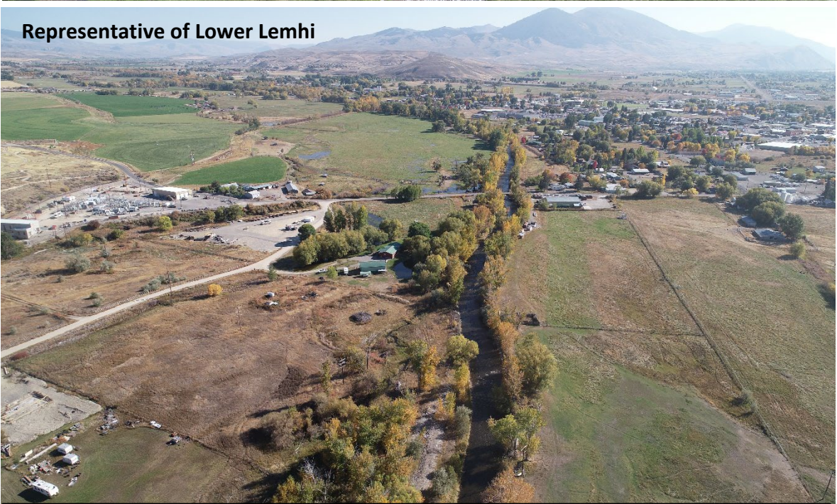
Representative photos of the upper and lower Lemhi River. Source: Daniel Bertram, Office of Species Conservation. The upper river (above) shows a meandering and more complex channel providing better spawning and fish-rearing habitat. In contrast, the lower river (below) shows a mechanically straightened channel—straightened in an attempt to minimize flooding of the adjacent agricultural and residential floodplain areas around the City of Salmon. This condition substantially reduced fish habitat.
