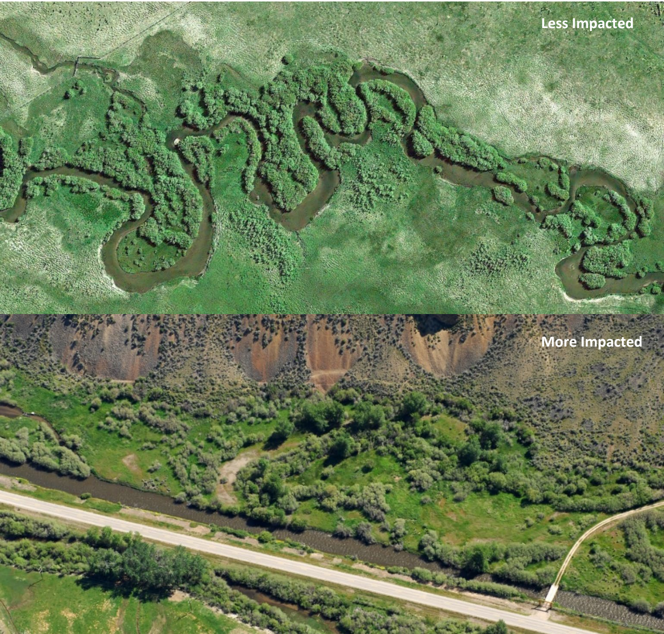
These examples of the Lemhi River above Hayden Creek illustrate the difference between a lesser manipulated reach that is influenced by groundwater and has a highly sinuous, multi-threaded channel with pools and narrow width-to-depth ratio stabilized by dense willow vegetation (top) and a more modified section that has been straightened during road construction. It is overly shallow and wide with plane-bed conditions (bottom). Flow is from right to left in both. Source: Reclamation
