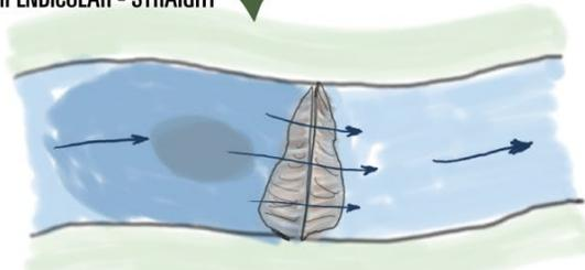
When dam crests span the bankfull channel, but are lower elevation than the adjacent floodplain, low flows are contained within the channel. Perpendicular orientations will back water up, and alter the flow paths to that of bankfull flows.
