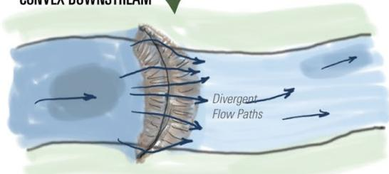
When dam crests are higher than bankfull and extend out onto floodplains, they can direct overflow onto those floodplains. However, a perpendicular, straight dam will
