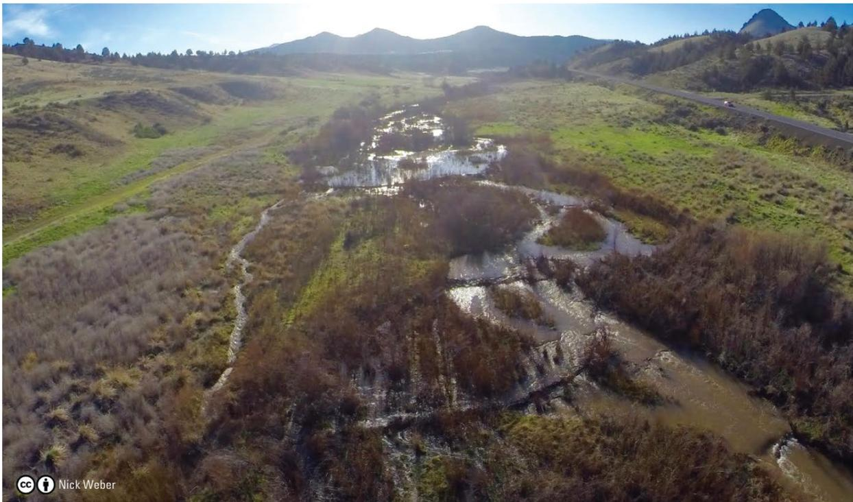
Figure 1 – The vision that guides the use of post-assisted log structures (PALS) and beaver dam analogues (BDAs) is ‘Stage 0,’ where large wood accumulation and beaver dams force the floodplain connectivity, multiple channels and complex physical instream and riparian habitat.
