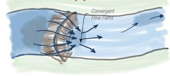
Beavers rarely build dams like Hoover Dam (and Hoover was not designed to withstand spill over the top). Concave downstream crests concentrate flow at the base of the dam, scouring out a deep pool, but also potentially undermining the dam integrity.
