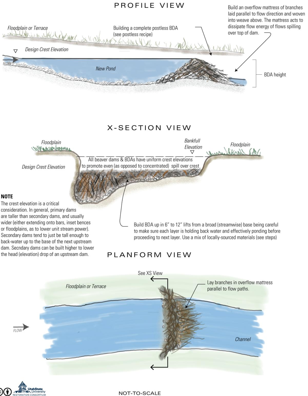
Figure 30 – Typical schematic sketches of a postless BDA.
