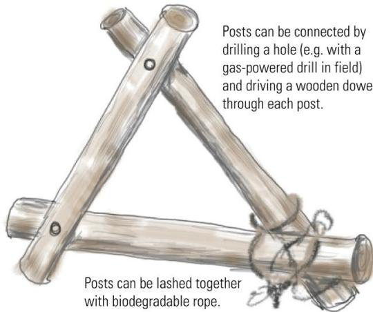
Posts can be connected by drilling a hole (e.g. with a gas-powered drill in field) and driving a wooden dowel through each post.
