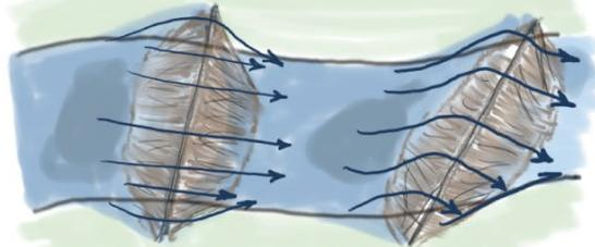
When dam crests are higher than bankfull and extend out onto floodplains, they can direct overflow onto those floodplains. However, a perpendicular, straight dam will direct most flow straight downstream. By contrast an angled dam will direct flow to one side of the channel (however the head drop tends to dissipate most of the flow energy).
