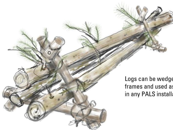
Logs can be wedged into triangle frames and used as key pieces in any PALS installation.
