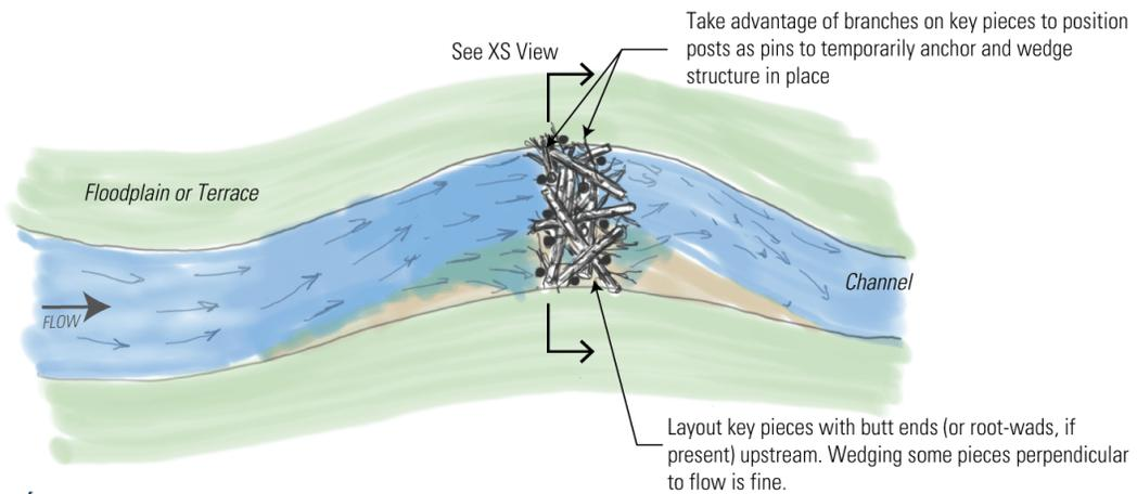
Take advantage of branches on key pieces to position posts as pins to temporarily anchor and wedge structure in place
