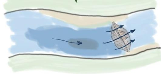
Smaller dams that just backup the low-flow channels often have an orientation perpendicular to the low flow, but at an angle to the bankfull flow patterns.
