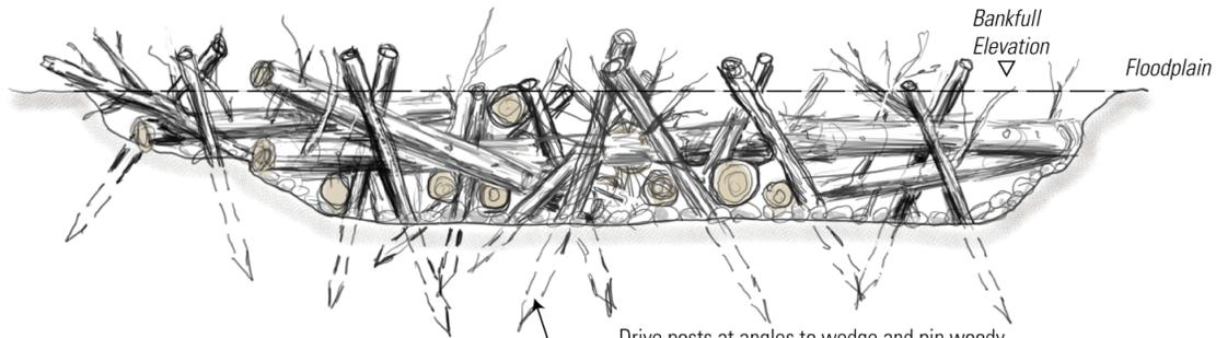
Drive posts at angles to wedge and pin woody debris together. Attempt to drive at least 1/4 to 1/3 of finished length of post into bed.
