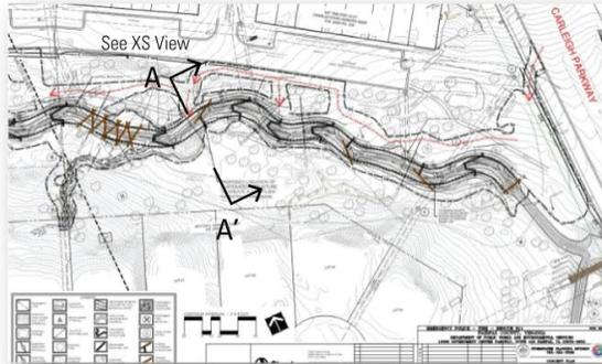
The plan tends to be overlaid on a topographic basemap, and shows specific locations of cross sections and/or profiles.
