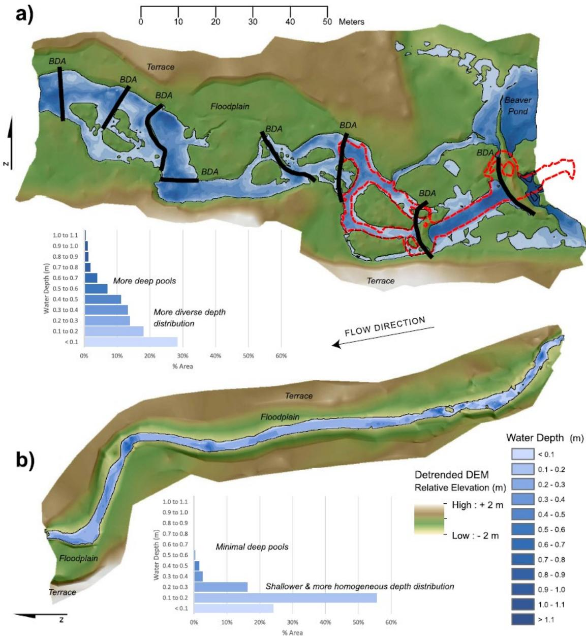
Figure 9 - Digital elevation models (DEMs) and water depth distributions for a A) typical reach with beaver dam analogues (BDAs) (i.e., successfully mimicking and promoting beaver dam activity) and B) without BDAs (i.e., structurally-starved control) from Bouwes et al. (2016b). Treatment area with BDAs has more channels and greater water depth variability than the control area without BDAs. Note: the red dashed line delineates the extent of a temperature experiment.
