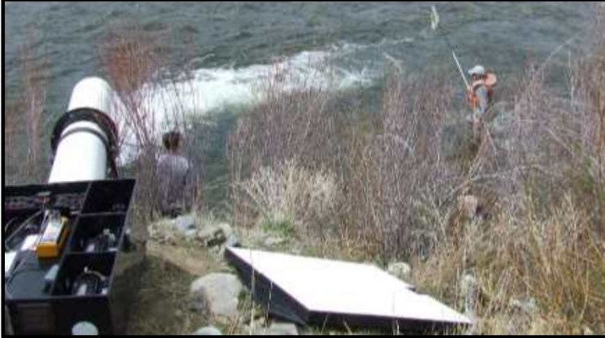
Photo 20. Biomark manufactured IS1001 PIT-tag detection systems were purchased in 2015 and are installed annually at the S-32 Diversion.
