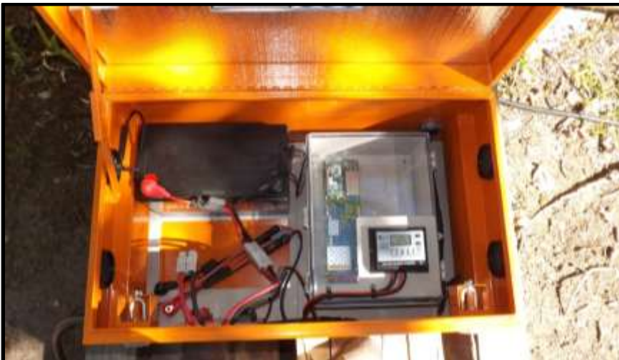
Photo 19. Biomark manufactured IS1001 PIT-tag detection systems were purchased in 2015 and are installed annually.
