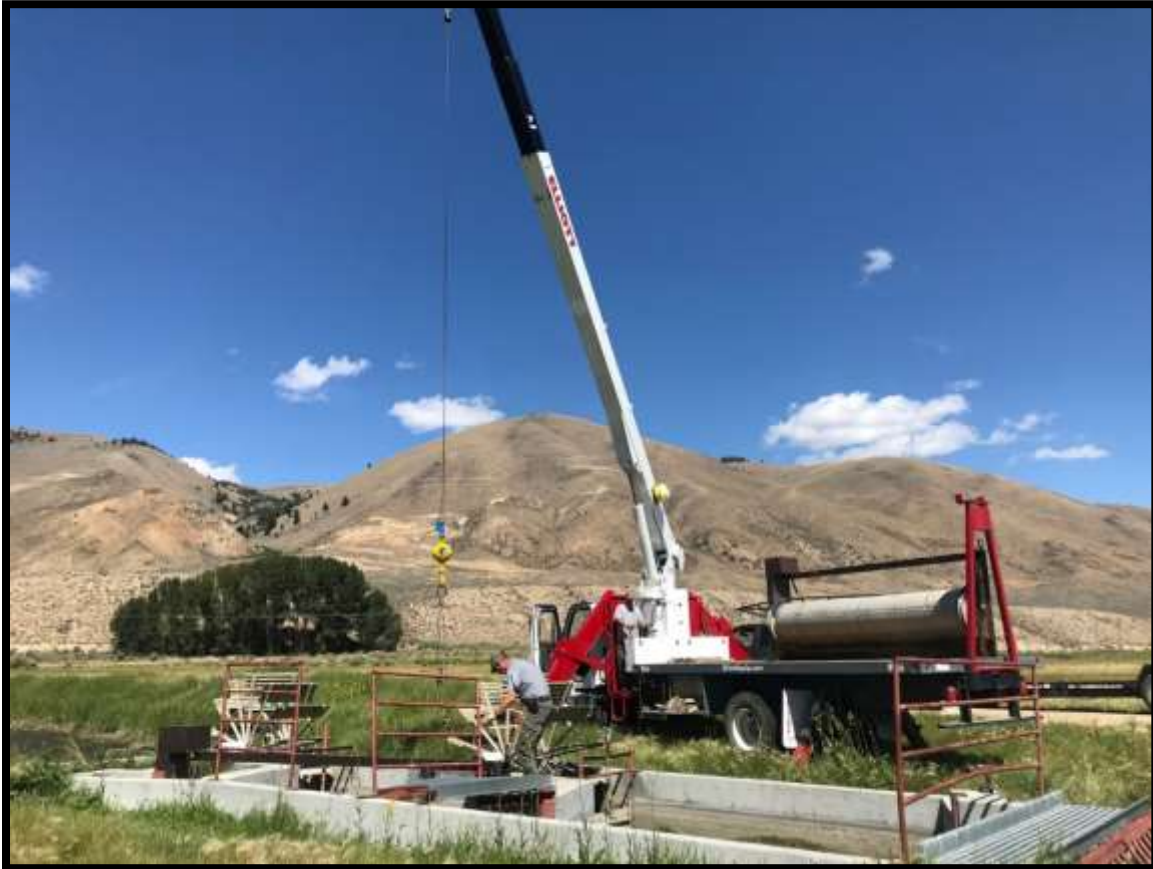
Photo 17. The Screen Program replaced a boom truck this year. The truck is used on a frequent basis to pull and set screens amongst other chores.
