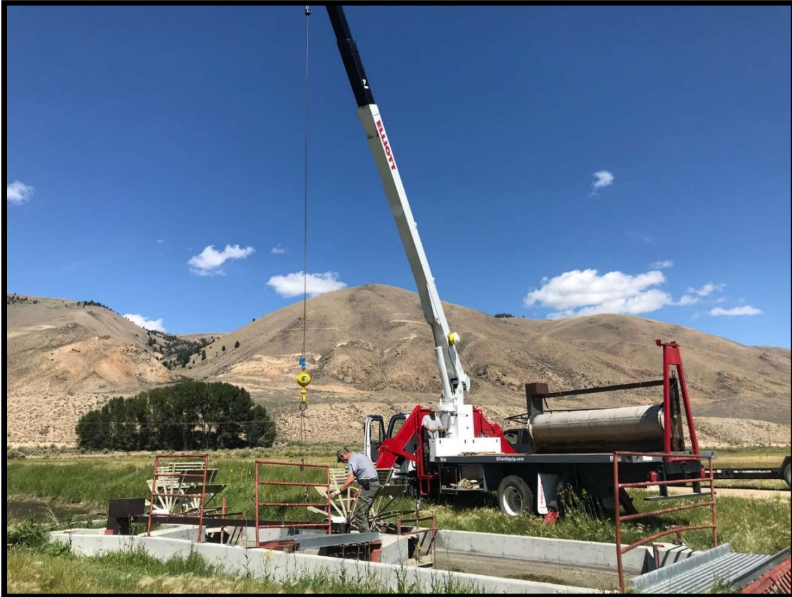
Photo 71. The Screen Program replaced a boom truck this year. The truck is used on a frequent basis to pull and set screens amongst other chores.
