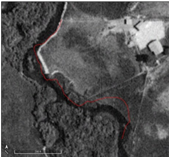
These GoogleEarth images from 1992 (left) and 2014 demonstrate the 50 feet of bank loss over time. The solid red line illustrates the bank line in 2014.
